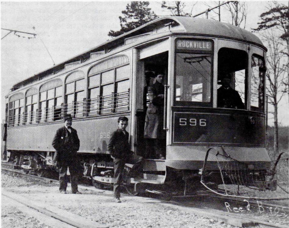
Leroy King describes this street car as one of Washington Railway's majestic "Rockville" cars, at 4 switch in 1908. Note multiple unit jumper box under center front window.
